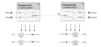
Use the **Sequence Viewer** tool to visualize events that represent the flow of messages, functions calls, and state transitions. To activate event logging, on the **Simulation** tab, in the **Prepare** section, select **Log Events**. To visualize the logged events, go to the **Review Results** section and select the Sequence Viewer.
