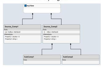
The hierarchy diagrams show a single root, which is the view specification. The root corresponds to the containing system box shown in the component view. The lines between components originate from the parent component with the filled diamond symbols that are used in UML compositions and end with a terminating dot at the child component.
